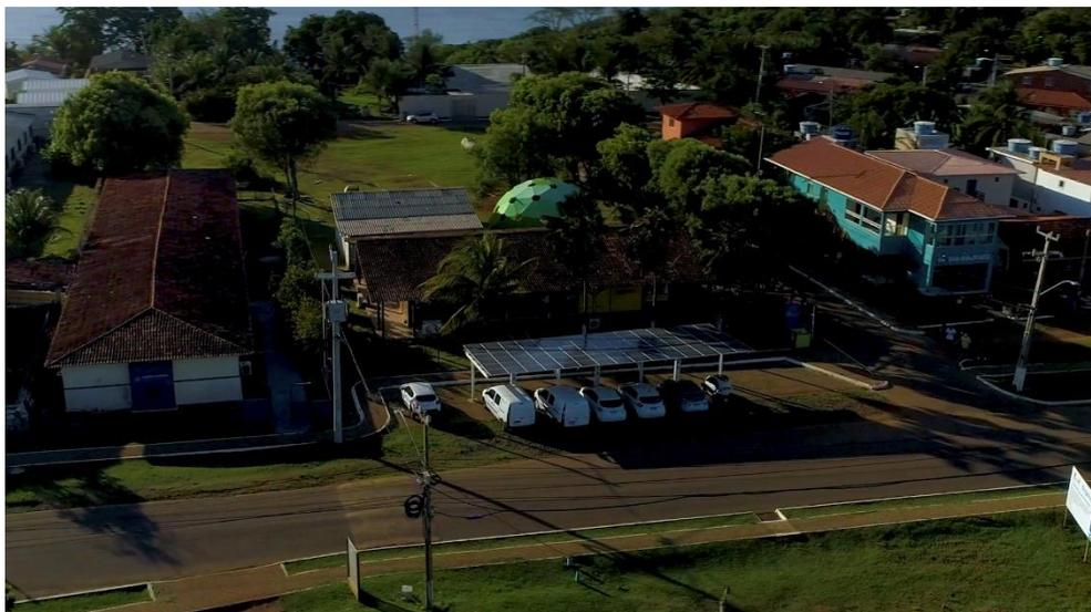
Each station can power up to six vehicles simultaneously and provides 26 MWh of energy per year. This energy generated is equivalent to 180,000 emission-free kilometres travelled, replacing about 20,000 litres of fossil fuel. What's more, excess energy is sent back to the grid for use by the local community.
